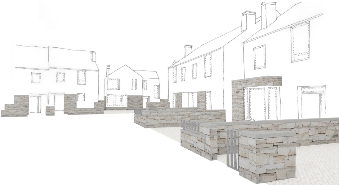
Fig. 41. Stone stitches house types together, provides a strong edge and robust face to heavily trafficked areas.
