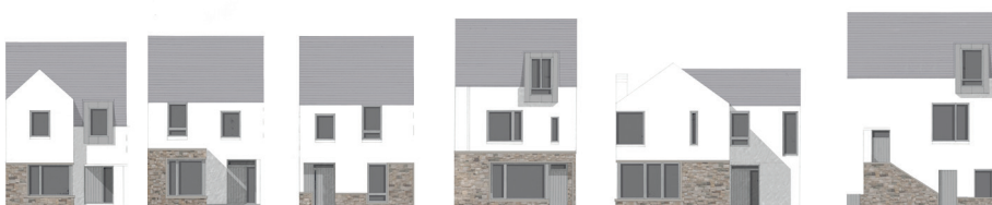
Fig. 42. Extent of stone facing to house types.
